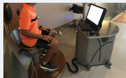
Figure 4: Athlete using the Balance Trunk MF system for assessment of Pelvic Stability.
