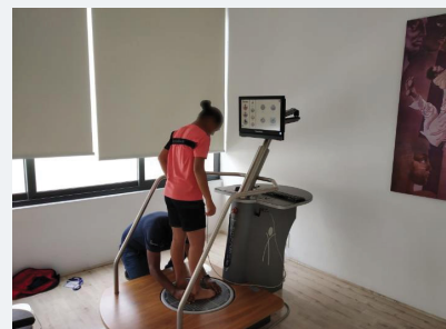
Figure 3: Athlete using the Prokin 252N system for assessment of Static and Dynamic stability.
