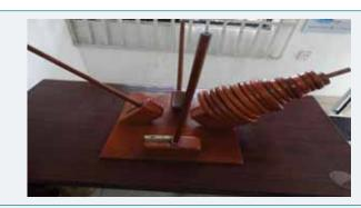
Figure 4: Eighteen pieces of circular wooden plates, ranging from 1.5 inches to 7.0 inches in diameter with a thickness of 0.5 inch.
