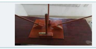
Figure 3: Four wooden poles, each having a length of 18 inches and a base of 3 inches that normally fit into the hole on the wooden block.
